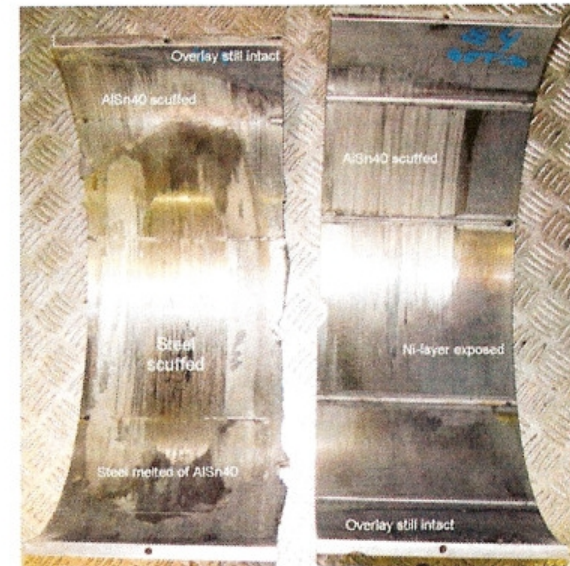
Overlayer completely corroded away, partly scuffing between Ni-layer and pin, partly steel-to-steel contact. Not acceptable.
